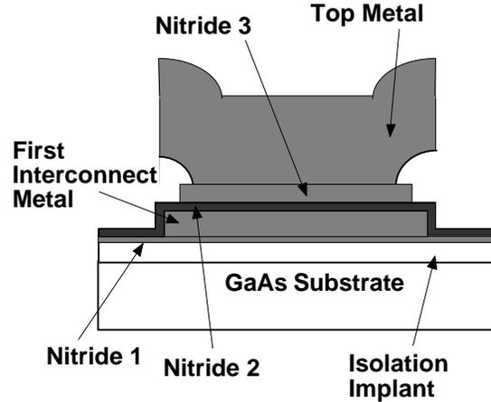
Fig. 1. Cross section of a MIMCAP.
