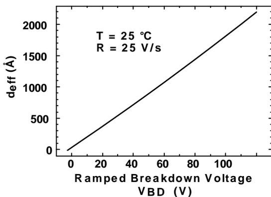
Fig. 3. Transformation from ramped breakdown voltage to nitride effective thickness.
