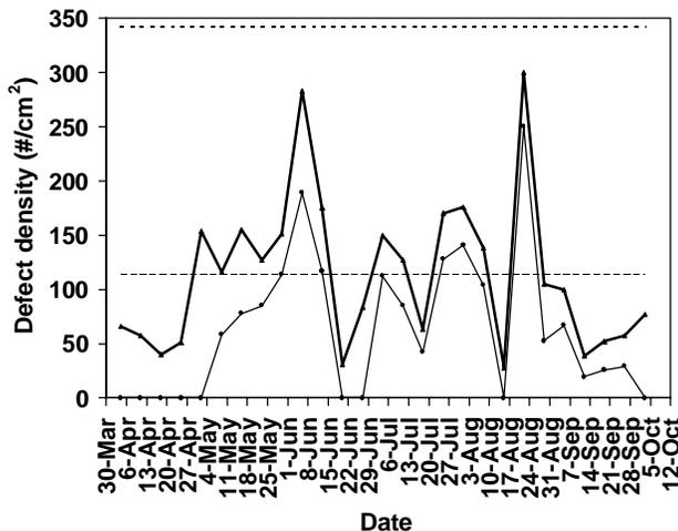
Fig. 7 Extrinsic defect density control chart.
