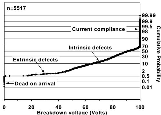
Fig. 5 Probability plot of approximately 5500 capacitors tested over a six month period.
