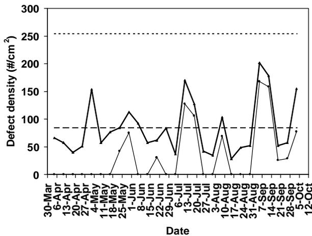
Fig. 6 Dead-on-arrival defect density control chart
