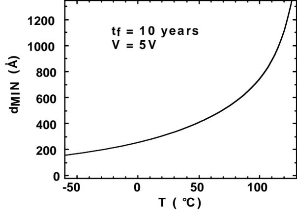
Fig. 2. Minimum effective thickness vs. temperature for a 10 year capacitor lifetime.
