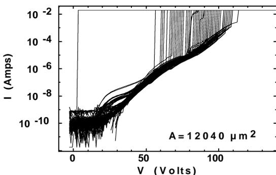
Fig. 4. IV characteristics of approximately 100 test capacitors.
