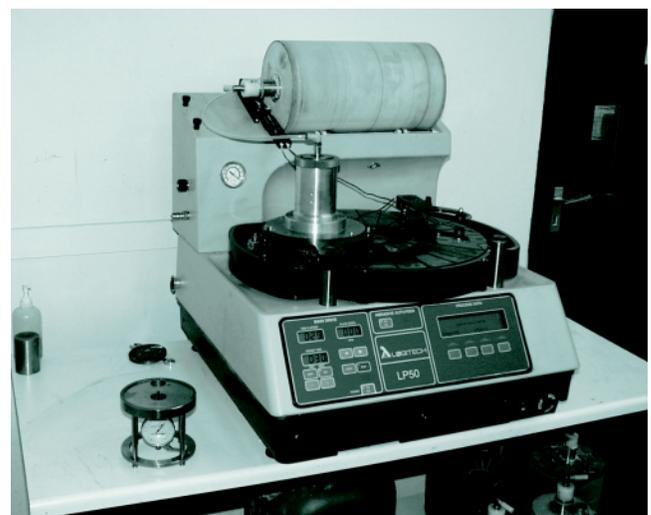
Figure 1: PP8GT lapping jig on LP80 lapping machine. Photo courtesy of Logitech Ltd.
