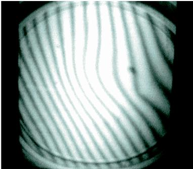
Figure 3: Interferogram of a bonded GaAs wafer after polishing
