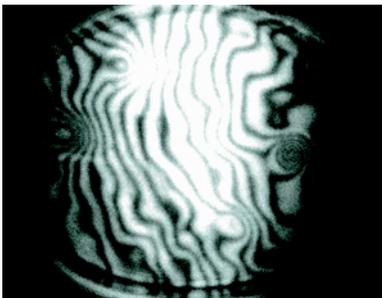
Figure 2: Interferogram of GaAs wafer after bonding, showing some localized high spots. Fringe spacing is 2 microns.
