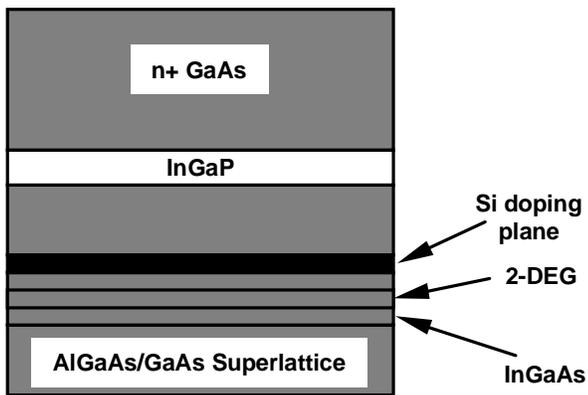
Figure 2 PHEMT layer structure with InGaP etch-stop
