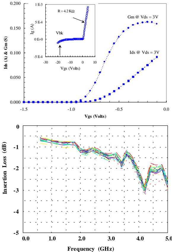
Fig. 2. Top panel: Transfer characteristics, showing a peak transconductance of 320 mS/mm; the inset plots the diode curve showing a breakdown  $V_{bk} > 20$  V. Bottom panel: RF insertion loss over 0.5–5 GHz in small signal S-parameter measurements for 30 PHEMT switches—10 unstressed samples and 20 HTRB stressed devices for 2,100 hours at 225 and 250°C.
