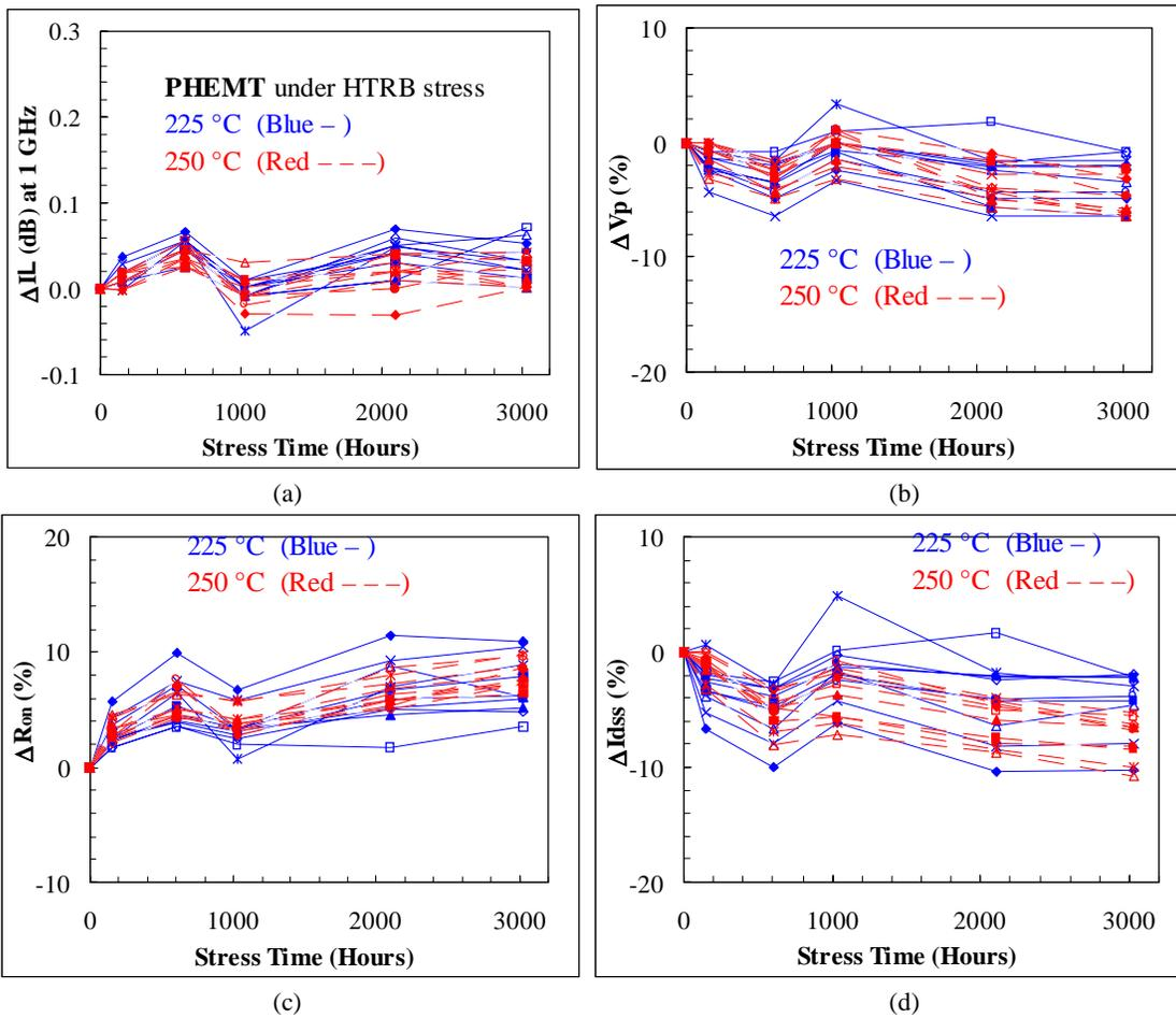
Fig. 4. Change of RF loss in dB and percentage change of primary DC parameters measured at room temperature over the elapsed HTRB stress at 225 (solid lines) and 250 °C (dashed lines): (a) Small-signal insertion loss at 1 GHz, (b) Pinch-off voltage, (c) Channel on-resistance, and (d) Drain saturation current.
