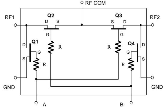
Fig. 1. PHEMT SPDT switch photograph and circuit schematics
