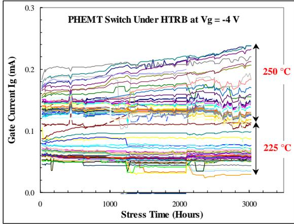
Fig. 3. *In-situ* gate current measured while devices (80 PHEMTs) were under HTRB stress at 225 and 250 °C.
