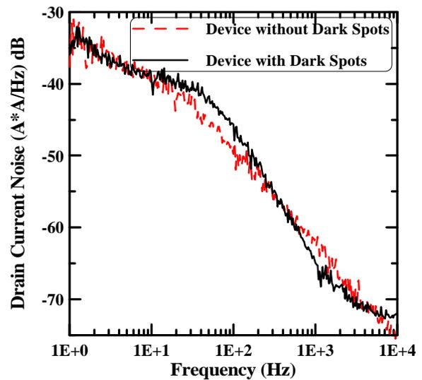
Fig. 8b Drain Current Flicker Noise Spectrum of Two Devices with and without Dark Spots
