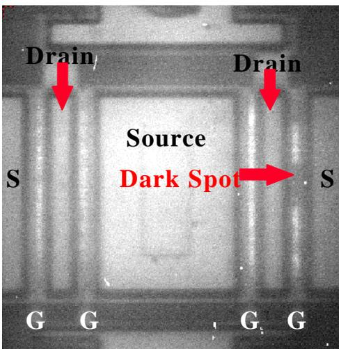
Fig. 8a Dark Spots of Light Emission at 1μm Found on One Finger
