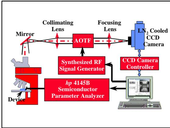
Fig. 1 Spectrally Resolved Imaging System
