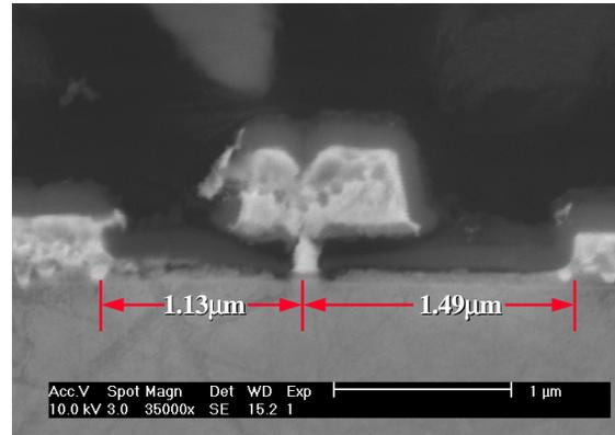
Fig. 6b Gate Misalignment of Device from Process # 1
