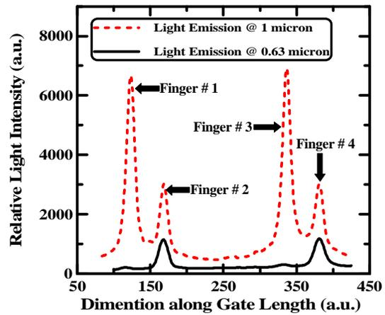
Fig. 4 Inhomogeneous Distribution of Light Intensity among 4 Fingers Showing Different Patterns at Different Wavelengths from Device of Process # 1
