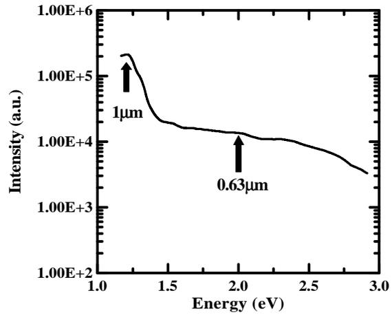
Fig. 2 Typical Spectrum of Light Emission from Power PHEMT
