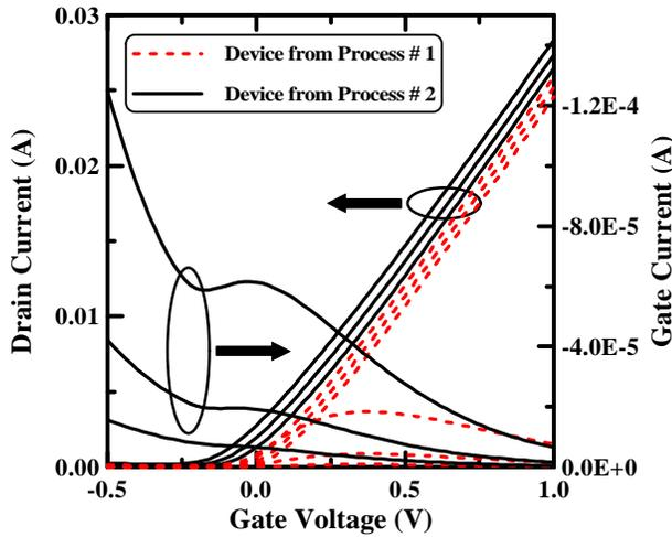
Fig. 3 Electrical Characteristics of PHEMT's from Two Processing Conditions
