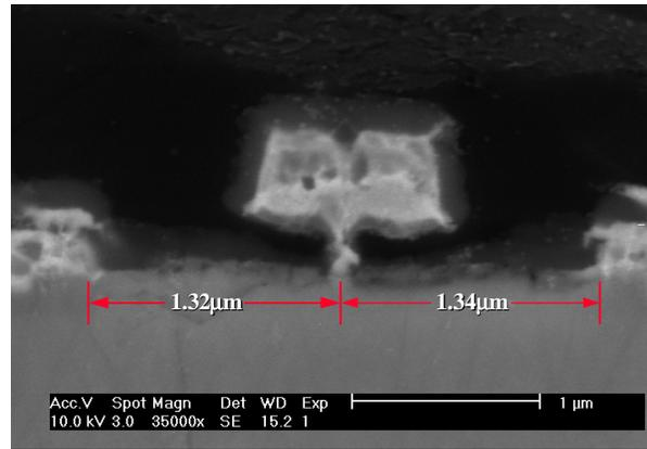
Fig. 7b No Gate Misalignment Found in Device from Process # 2
