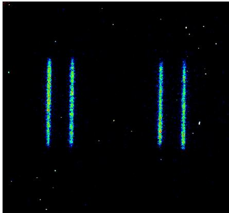
Fig. 7a Relatively Uniform Light Emission Distribution among 4 Fingers of Device from Process # 2
