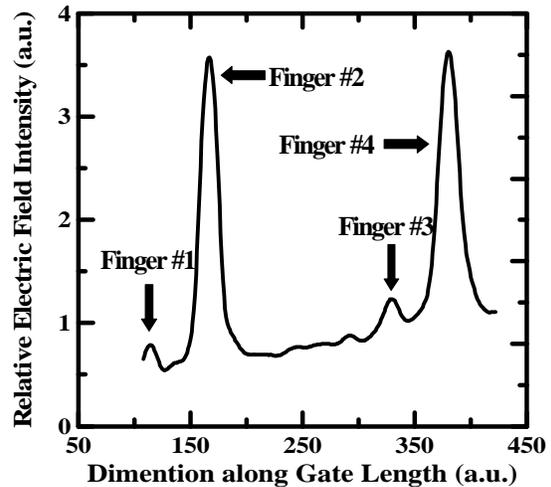
Fig. 5b Relative Maximum Electric Field Distribution among 4 Fingers
