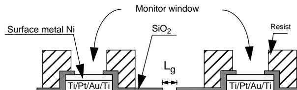
Fig. 1: Schematic view of wet-chemical recess etching for HFET fabrication.
