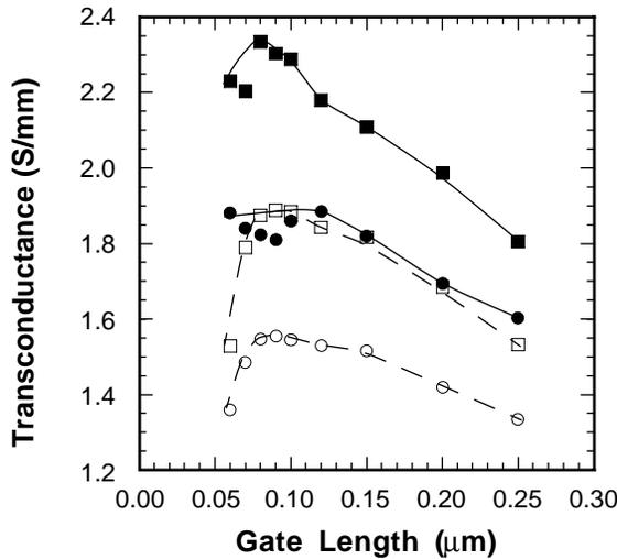
Fig. 4:  $g_m$  of HFETs with  $L_g$  ranging from 0.06 to 0.25  $\mu\text{m}$ . The experimental points, indicated with open and solid symbols, stand for devices with shallow and deep etching, respectively. Besides, the circles and squares are for the values measured at  $V_{ds}$  of 1 and 2 V.
