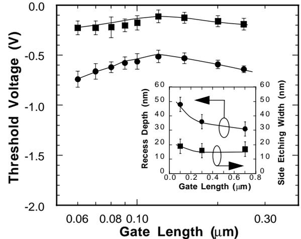
Fig. 3: Threshold voltage (measured at  $V_{ds} = 1.0$  V) of HFETs with  $L_g$  ranging from 0.06 to 0.25  $\mu\text{m}$ . The experimental points, indicated with circles and squares, stand for devices with shallow and deep etching, respectively. The inset shows the variations of recess depth and side etching that are induced by the change in gate length.
