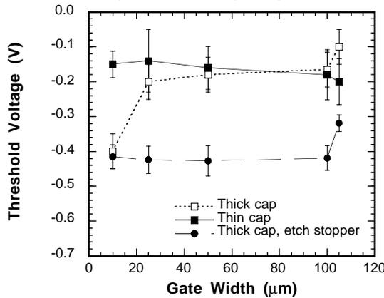
Fig. 2: Threshold voltage versus the total gate width of 0.1- $\mu\text{m}$  HFETs. The  $W_g$  of 10, 25, 50, 100, and 105  $\mu\text{m}$  corresponds to with gate layouts of  $1 \times 10$ ,  $2 \times 12.5$ ,  $2 \times 25$ ,  $2 \times 50$ , and  $4 \times 25 \mu\text{m}$ , respectively.
