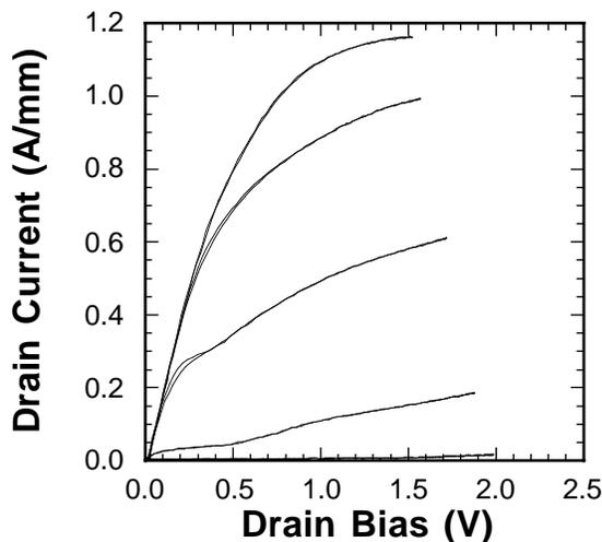
Fig. 6: I-V characteristics of D-MODFETs (a) and E-MODFET (b) with a gate periphery of 0.03  $\mu\text{m} \times 100 \mu\text{m}$ . The  $V_{gs}$  for the top curves is 0.8 V, and the measurement step of  $V_{gs}$  is 0.2 V.
