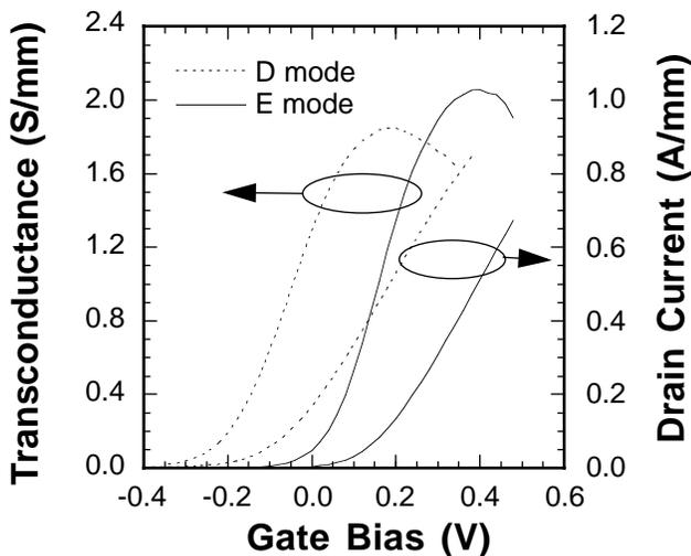
Fig. 5: Transfer characteristics for a 0.03- $\mu\text{m}$  gate length D-MODFET (dashed lines) and a 0.03- $\mu\text{m}$  E-MODFET (solid lines). The devices were biased at  $V_{ds} = 1.0$  V.
