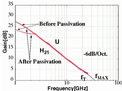
Fig. 5 Comparison of the microwave performance before and after passivation for a 2x10μm<sup>2</sup> single emitter device
