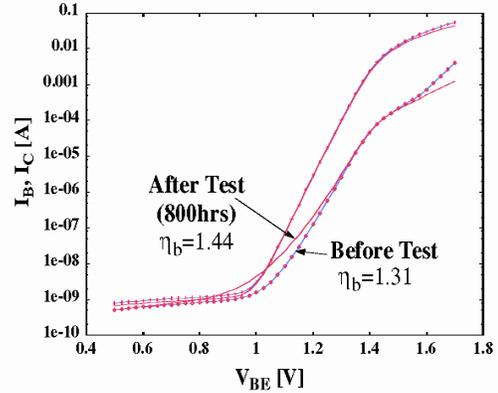
Fig. 6 Gummel plot of passivated 2 finger 5x10μm<sup>2</sup> emitter HBTs before and after long term reliability tests.
