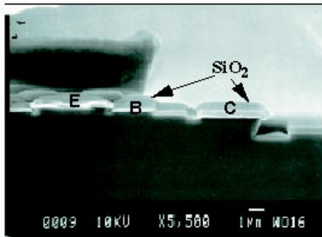
Fig. 4 Cross section of passivated GaInP/GaAs HBTs with PECVD SiO<sub>2</sub>(4500Å)
