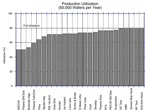
Fig. 4 - Equipment Utilization of a Production Wafer Fab
