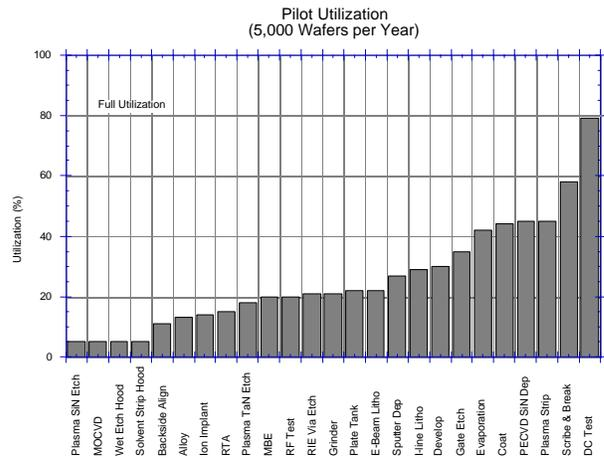
Fig. 3 - Equipment Utilization of a Pilot Wafer Fab
