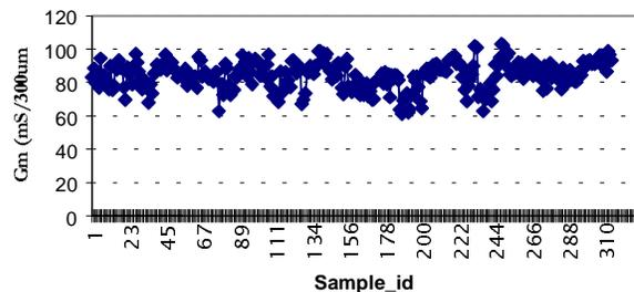
Figure 2: RF Gm Trend for PWRPHEMT Devices Measured at Standard Bias Conditions
