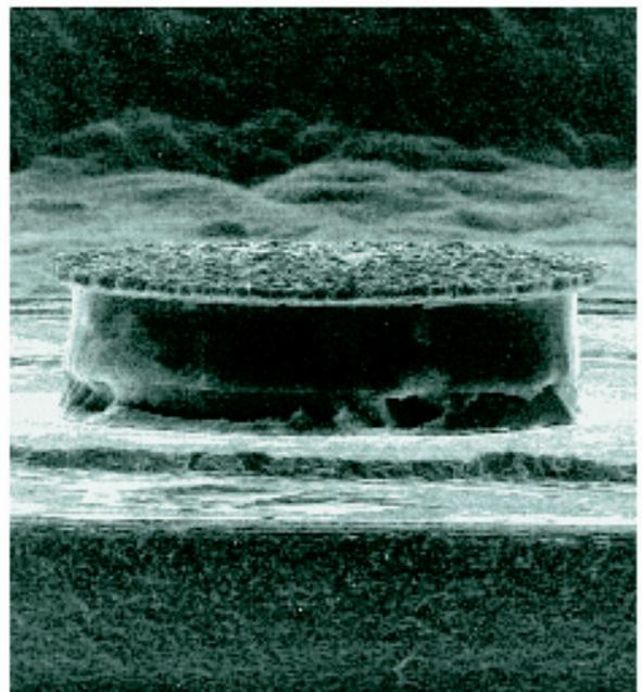
Fig. 2: SEM of  $\text{FeCl}_3$  wet etched InP 77 GHz Gunn diodes.
