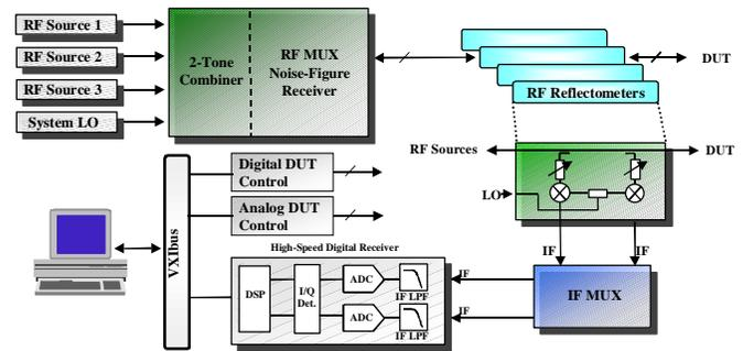
Figure 3. High-level System Block Diagram.
