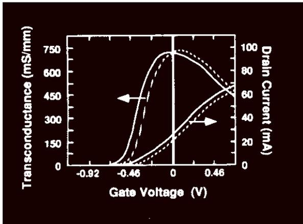
Fig. 5. Typical effects of hydrogen exposure to PHEMTs before (—) and after (---) exposure to 4%  $H_2$  for 10 min at 270C (after [6]). In some applications, the design current and transconductance can be recovered by re-biasing the device.
