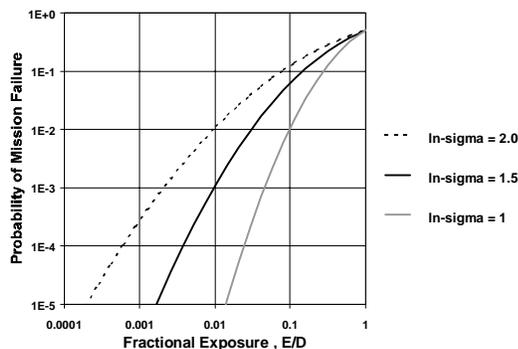
Fig. 1. Failure probability versus fractional dose for various log normal standard deviation values
