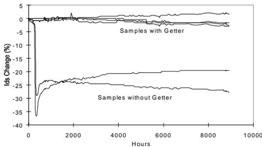
Fig. 4. Lifetest data comparing  $I_{DSS}$  of GaAs PHEMTs in gettered and ungettered packages. The getter was designed for a 15 year mission life at 125C
