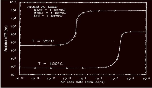
Fig. 3. Modeled MTTF of a hermetically packaged PHEMT versus package leak rate; results for two different package temperatures are shown.
