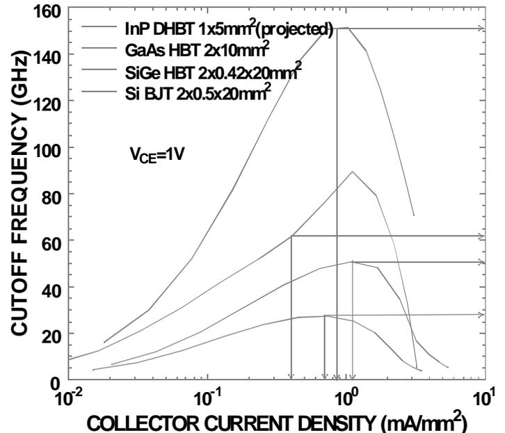
Figure 2: Cutoff Frequency ( $F_t$ ) for a selection of bipolar technologies
