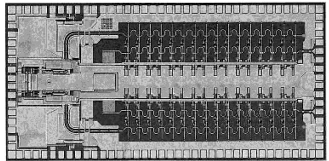
Figure 7: Microphotograph of GaAs 10GB/s modulator driver chip
