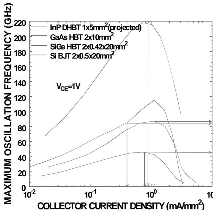
Figure 3: Maximum Oscillation Frequency ( $F_{max}$ ) for a selection of bipolar technologies
