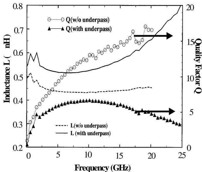
Figure 4: Inductance and Q factor for an example silicon-based spiral inductor
