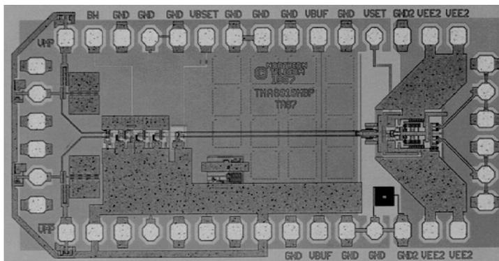
Figure 6: Microphotograph of SiGe 10GB/s limiting amplifier chip
