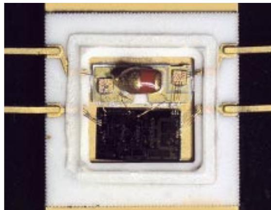
Figure 4: De-lidded Ku-band module.
