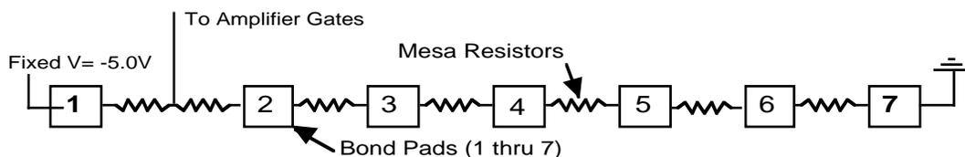
Figure 1: On chip resistor network used to bias all MMIC stages.
