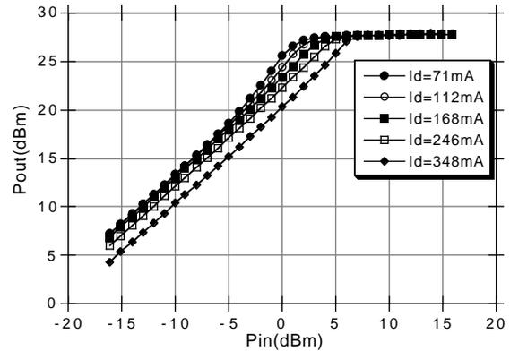
Figure 3: Pout versus Pin as a function of Ids.
