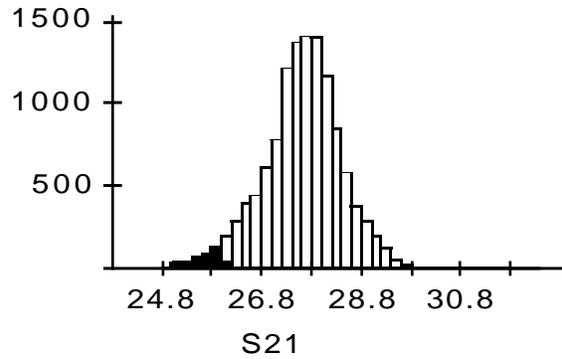
Figure 6: On wafer gain histogram. Highlighted region has gain < 26dB.
