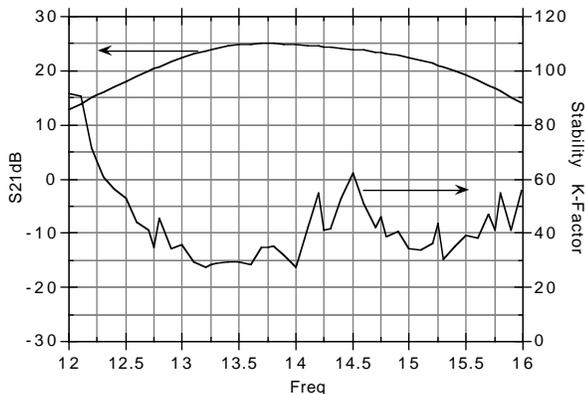
Figure 2: S21 and Stability K-factor versus frequency.
