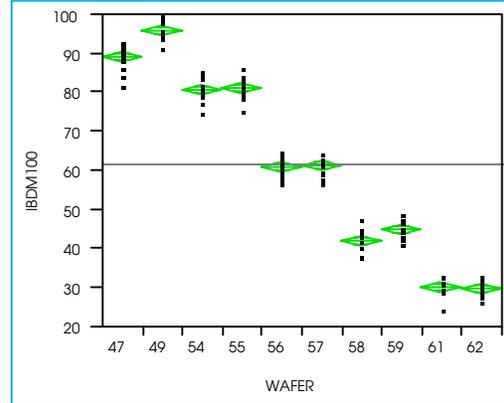
Figure 2- Dose split across the process spec window. Here wafers were implanted with a separate dose to induce a current ( $I_{dss}$ ) split on depletion FETs.
