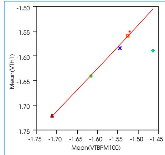
Figure 4- Threshold voltage of the individual power FETs correlated to the DC threshold voltage measured at unit probe.  $R^2=0.994$
