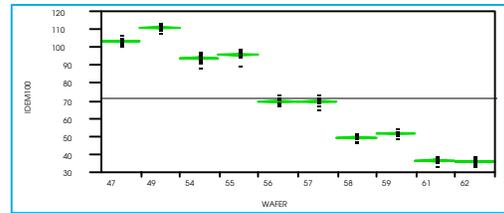
Figure 3- Dose split across the process spec window. Here wafers were implanted with a separate dose to induce a current ( $I_{dss}$ ) split on enhancement FETs.
