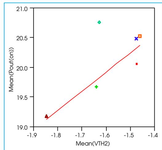
Figure 5- Output power in RF correlated to the DC threshold voltage measured at unit probe.  $R^2=0.9$
