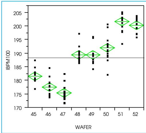
Figure 1- Dose split across the process spec window. Here wafers were implanted with a separate dose to induce a current ( $I_{dss}$ ) split on power FETs.
