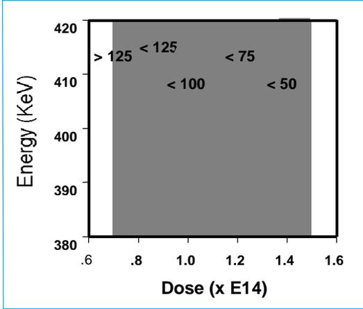
Fig 1. Contour plot of isolation resistance as a function of He++ ion dose and implant energy.
