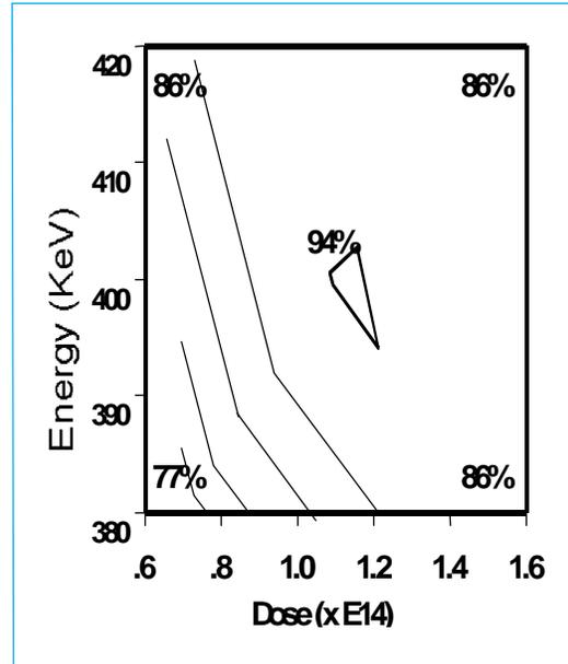
Fig 2. Package yield of 5V, 1.9Ghz HBT amplifier chip as a function of He++ dose and implant energy.
