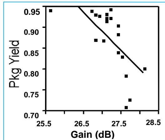
Figure 3. Final package yield of 5V, 1.9Ghz amplifier vs. amplifier gain.
