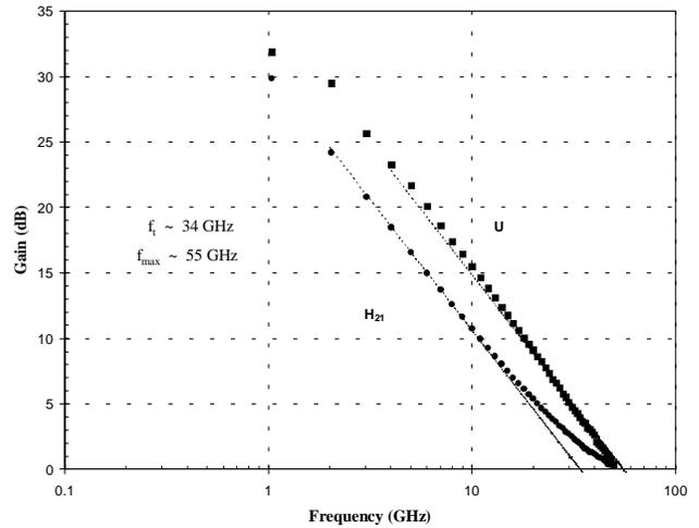
Fig. 5. RF results from a  $1.4 \times 3 \mu\text{m}^2$  device on the 35% AlGaAs structure. The extrapolated  $f_i$  and  $f_{\text{max}}$  are 34 and 55 GHz. The measurements were taken at  $V_{\text{ce}} = 1.5 \text{ V}$  and  $I_{\text{c}} = 2 \text{ mA}$ .
