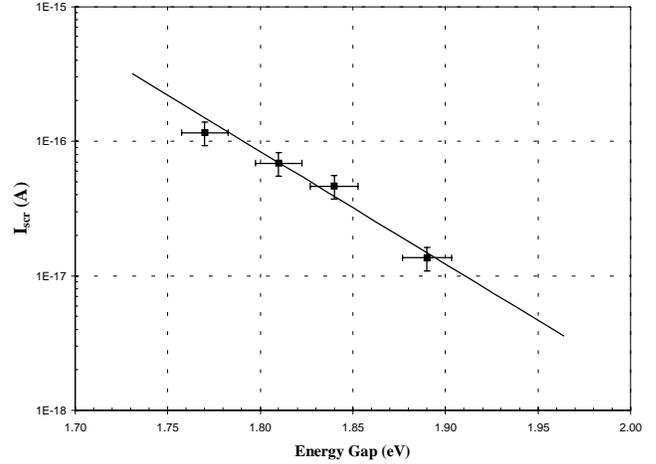
Fig. 2. Extrapolated space charge recombination component of the base current ( $I_{b1} = I_{scr} \exp(qV_{be}/2kT)$ ) as a function of the energy-gap of the AlGaAs in the emitter. The solid line is a fit to the data assuming the basic expression for  $I_{scr}$  found in the text.
