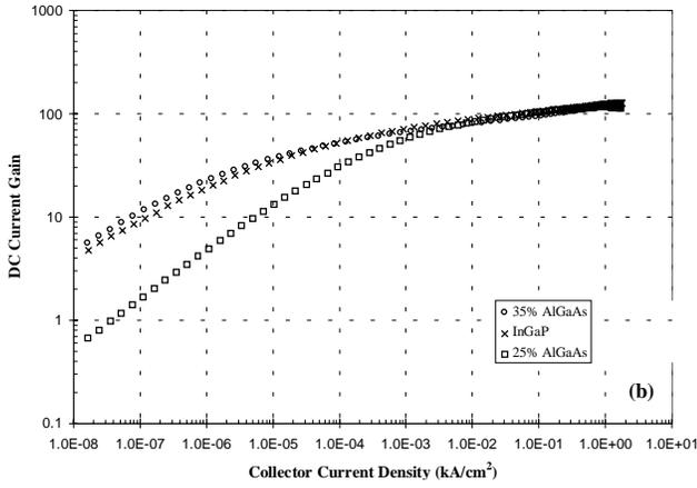
Fig. 1. Gummel plots (a) and DC current gain versus current density curves (b) from large area devices ( $75 \times 75 \mu\text{m}^2$ ) on three samples with different emitter structures and  $4 \times 10^{19} \text{ cm}^{-3}$  base layers ( $R_B \sim 250 \Omega/\square$ ). Note the base current at low injection levels ( $V_{be} < -0.9 \text{ V}$ ) for the 35% AlGaAs emitter is nearly an order of magnitude lower than the 25% AlGaAs structure and comparable to the InGaP emitter.
