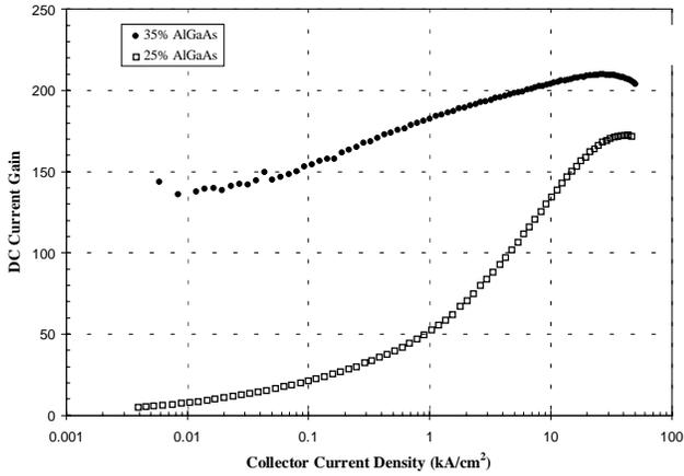
Fig. 3. Gain versus current density from small area devices ( $1.4 \times 3 \mu\text{m}^2$ ) on two wafers with different Al composition in the emitter. The gain at low current density is significantly improved with the higher energy-gap emitter.
