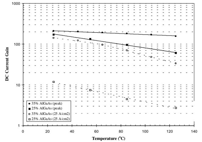
Fig. 4. Dependence of DC current gain on temperature in small area devices ( $1.4 \times 3 \mu\text{m}^2$ ) on two wafers with different Al composition in the emitter. The solid points are for peak gain, the open points for the gain at a fixed collector current density of  $25 \text{ A/cm}^2$ . The line are exponential fits to the data used as a guide for the eye.
