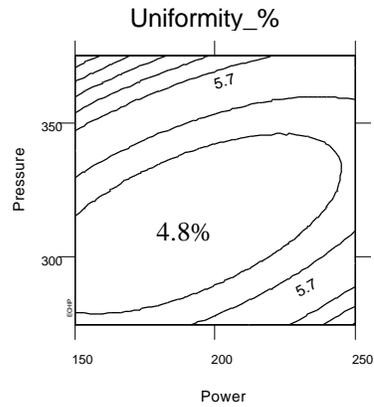
**Figure 2: 2<sup>nd</sup> CCC Experiment etch Uniformity**
