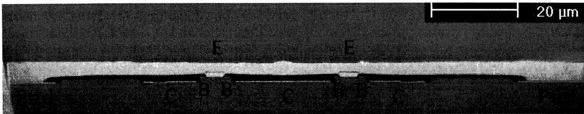
Figure 1. HBT cross section showing a polyimide planar process with MeV Implant isolation
