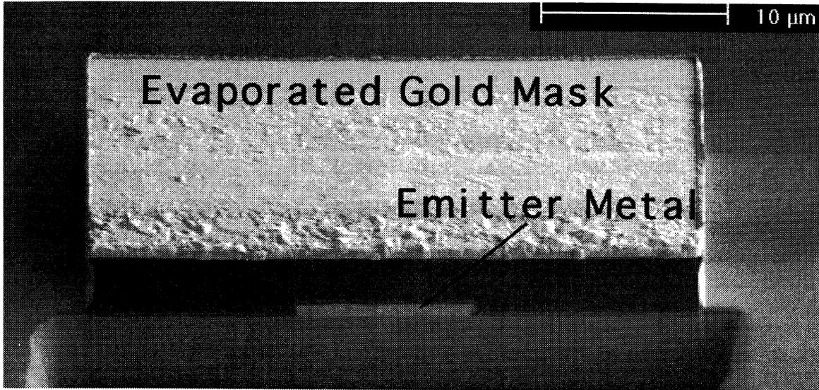
Figure 3. Original Implant Mask using photoresist and evaporated gold
