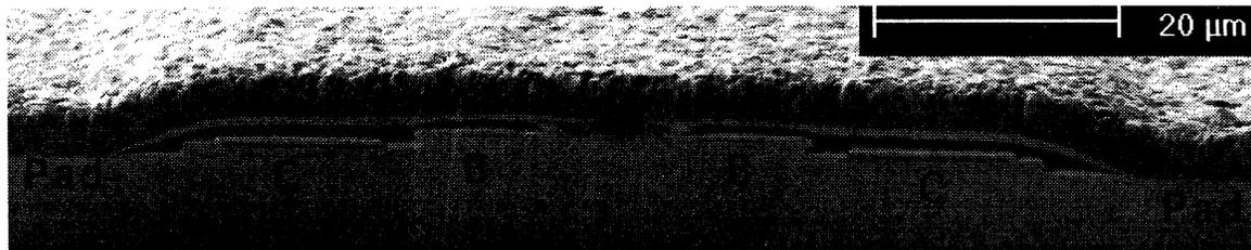
Figure 2. HBT cross section showing a full mesa isolation process with air-bridge
