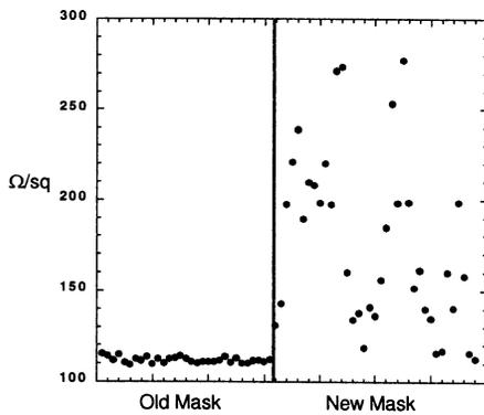
Figure 4. Sheet resistance data for the emitter TLM using base metal contacts
