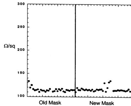
Figure 5. Sheet resistance data for the emitter TLM using Emitter metal contacts
