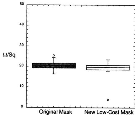
Figure 6. Emitter layer sheet resistances from sister wafers using, old and new masking schemes
