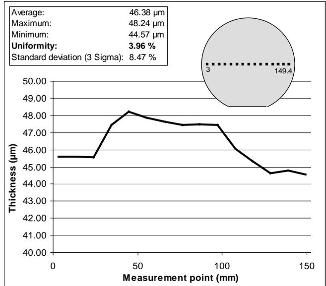
Fig. 3: Results on wax coating of 6'' GaAs wafer: thickness uniformity
