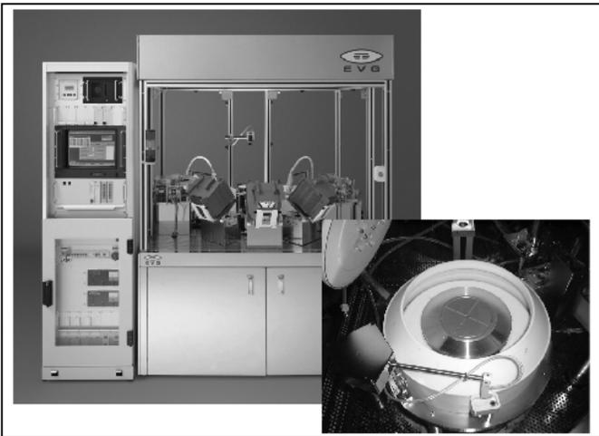
Fig. 1: Wax Bonder with coating module and heatable chuck
