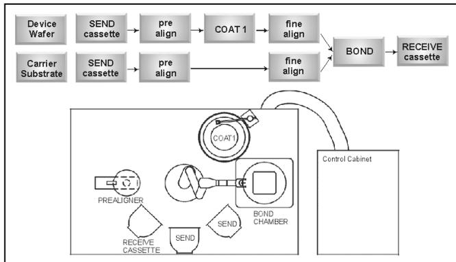
Fig. 2: Process flow for automatic wax coating and bonding and schematic top view of the Wax Bonding System
