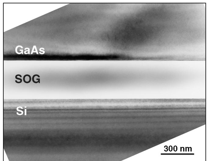
Fig. 6: Cross sectional TEM image of the GaAs/SOG/Si ComBond wafer interface
