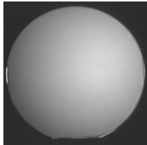
Fig. 5: IR transmission image of a GaAs/SOG/Si ComBond wafer after annealing at 200°C/10 h
