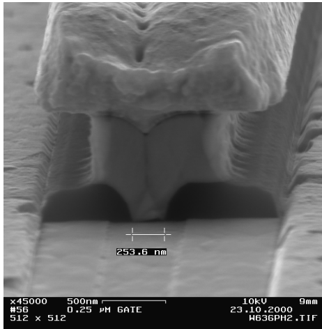
Fig.1 : SEM picture of cross section of the 0.25 μm gate.
