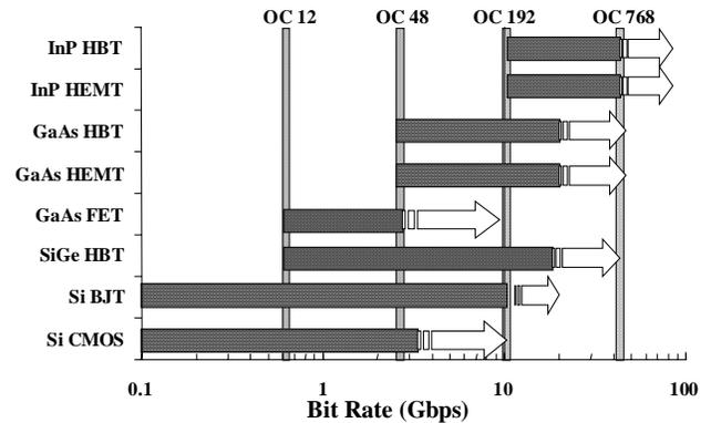
Figure 3 High speed ASIC technology for several generations of lightwave communication ASICs.
