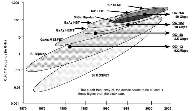
Figure 2 Semiconductor technology roadmap for lightwave electronics.
