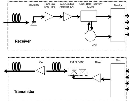
Figure 1 The schematic diagram of a generic opto-electronic transceiver.
