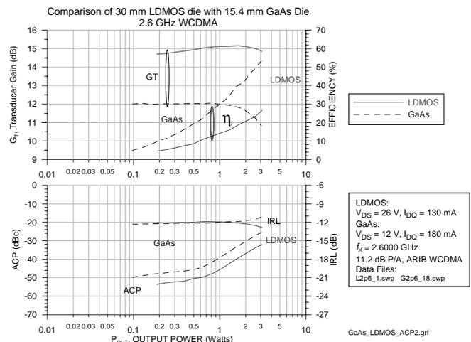
At lower frequencies, the linearity vs. efficiency gap narrows. Power GaAs transistor efficiency (at 2.1GHz) is on par with LDMOS or at best, up to 5% better in efficiency than LDMOS. This depends greatly on the required ACP
