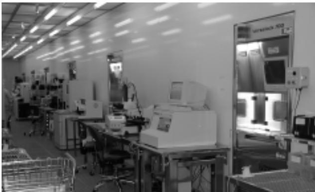
Figure 2. Etch bay populated multi-chamber ICP etch tools.
