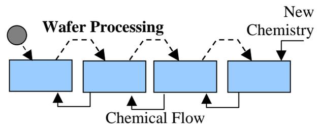
Figure 4: Flow of Wafers and Solvents for the Demount Process
