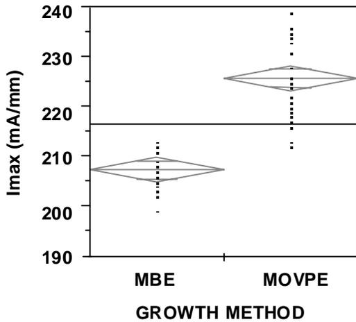
Fig. 2.  $I_{max}$  versus growth method.
