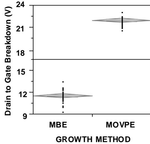
Fig. 3. Drain to gate breakdown versus growth method.
