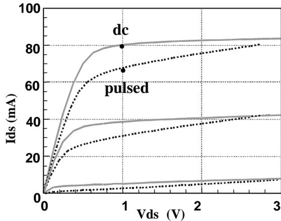
Fig. 6. dc versus pulsed IV for MBE (ratio 0.81)
