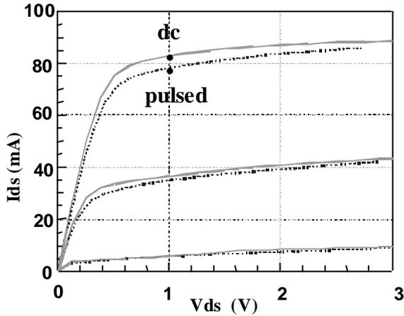
Fig. 5. dc versus pulsed IV for MOVPE (ratio 0.91)
