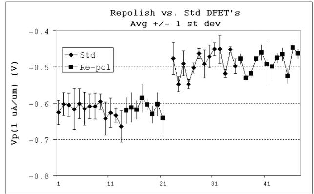
Fig. 5 Depletion Mode FET Pinchoff Voltage Results
