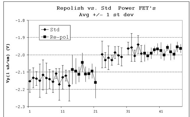
Fig. 6 Power FET Pinchoff Voltage Results
