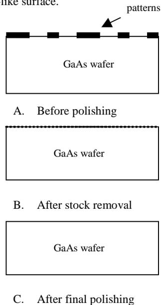
Fig. 1 Schematic representation of GaAs wafer polishing sequence
