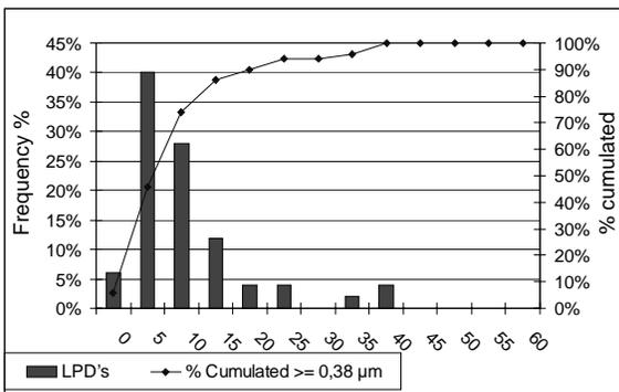
Fig. 2 LPD's frequency and cumulative LPD's at 0.38  $\mu\text{m}$  (Surfscan 5500)
