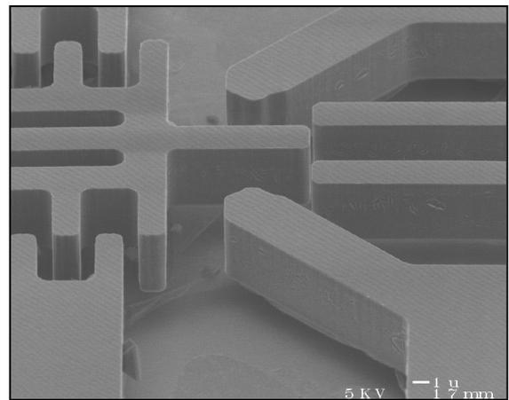
Figure 2 Scanning electron microscope view of the switch
