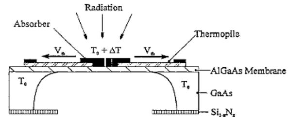
Figure 4 Cross section of an AlGaAs-based infrared bolometer [14]
