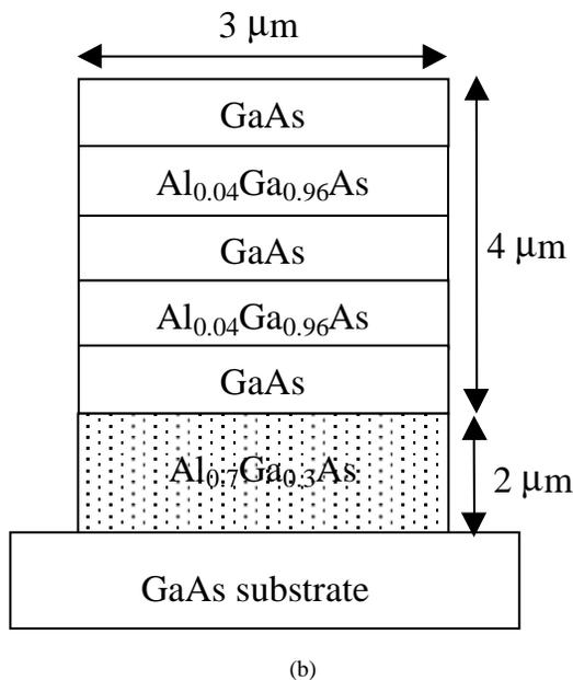
Figure 1 (a) Schematic top view of the 1x2 waveguide switch (b) Cross sectional view of the layer structure comprising the waveguide. Shaded area indicates sacrificial layer
