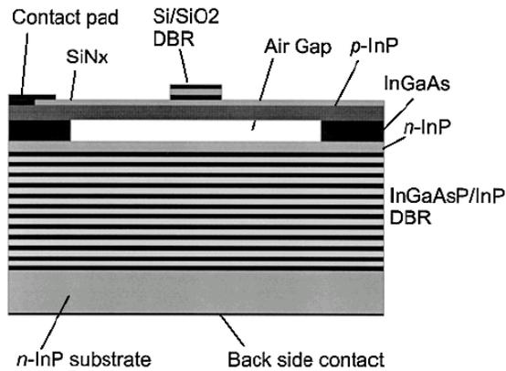
Figure 2 Schematic cross section of InP-based tunable Fabry-Perot filter [11]
