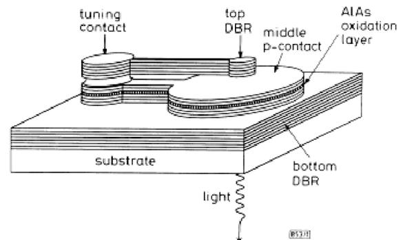
Figure 1 Schematic diagram of a micromechanical tunable VCSEL [7]
