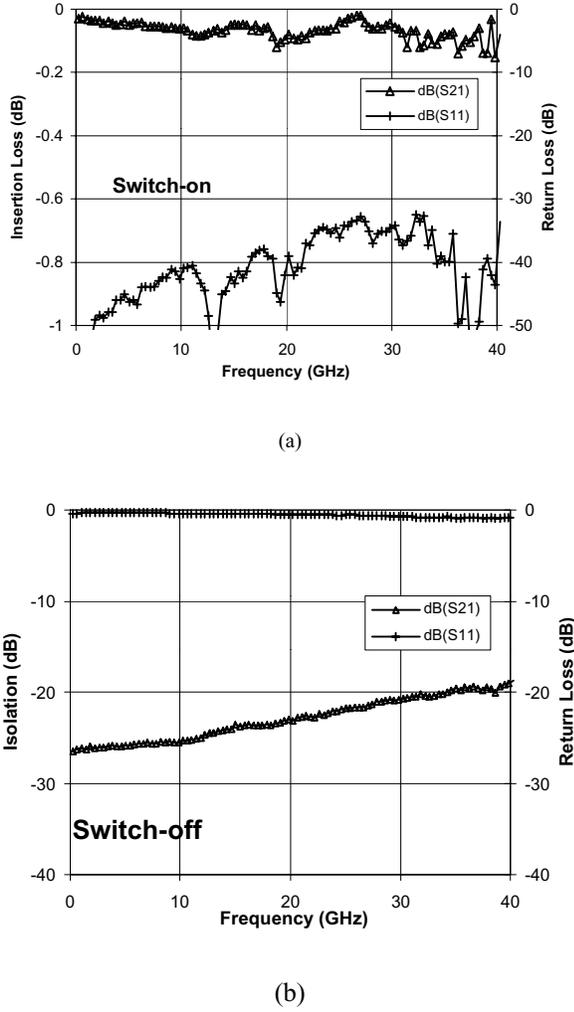
Figure 3. The measured RF performance of cantilever switches for (a) switch-on and (b) switch-off states
