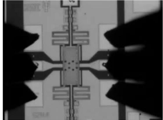
Figure 2. A microscope picture of a cantilever switch
