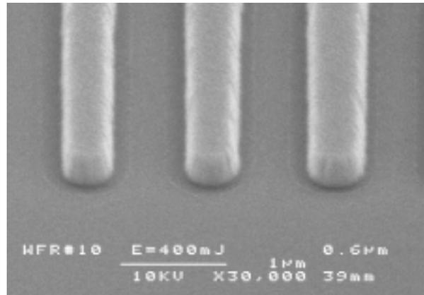
Figure 4. Equal line-space 0.6µm metal lines following lift-off.
