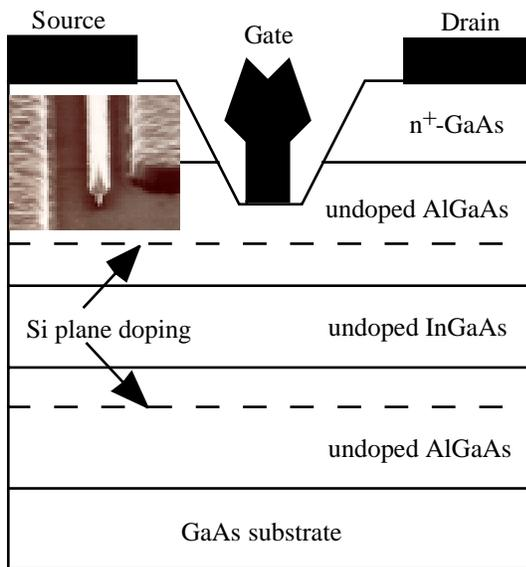
Fig.1: Cross section of an AlGaAs/InGaAs power HEMT (Insert: 0.1 μm T-gate).
