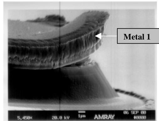
**Figure 6 - Metal Encapsulated**
