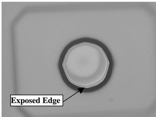
**Figure 5 – Inadequate Resist**
