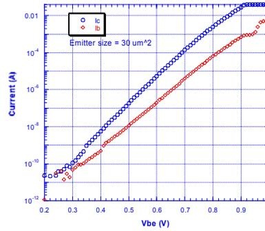
Fig. 4 A gummel plot of a SHBT with  $4E19\text{ cm}^3$  base doping
