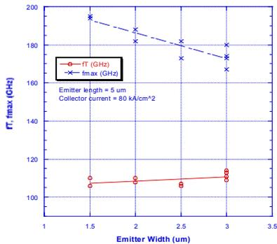
Fig. 3  $f_T$  and  $f_{max}$  plot against the emitter stripe widths
