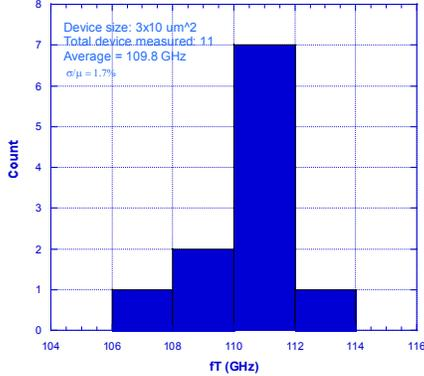
Fig. 2 A histogram of  $f_T$  on  $3 \times 10\text{-}\mu\text{m}^2$  HBTs across a 2-inch wafer
