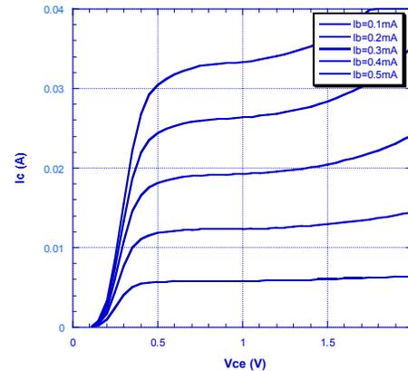
Fig. 1 A typical I-V curve for a hexagonal- $3 \times 10 \mu\text{m}^2$ -emitter HBT
