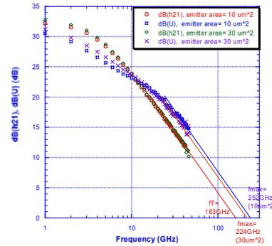
Fig. 5 A plot of  $|h_{21}|$  and  $U$  for  $3 \times 10\text{-}\mu\text{m}^2$  and  $2 \times 5\text{-}\mu\text{m}^2$  SHBTs. The S-parameters are measured from 0.25 GHz to 40 GHz
