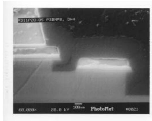
Figure 2 (b): A blowup of emitter and base contact area of the InP HBT device shown in figure 2 (a).
