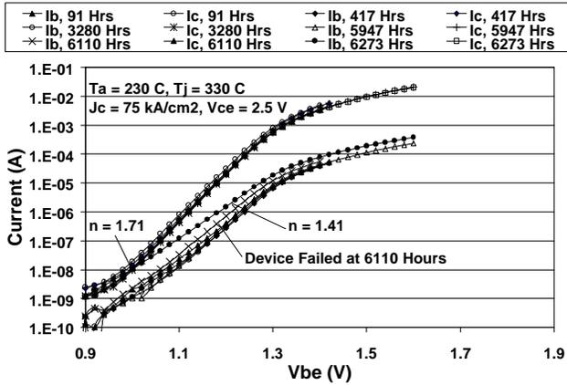
Fig. 4. Gummel plots of a  $2 \times 12 \mu\text{m}^2$  InGaP HBT measured at different stages of traditional low current stress test in oven. The stress current density was  $75 \text{ kA/cm}^2$ .
