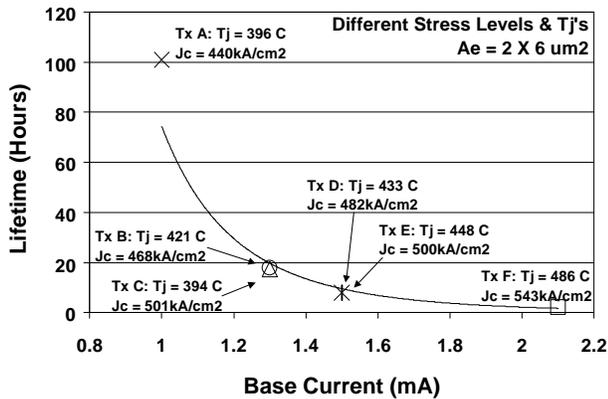
Fig. 6. Lifetimes of InGaP HBTs plotted as a function of applied base currents.
