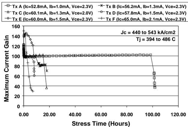
Fig. 2. Changes in peak room-temperature gain over stress time for the transistors listed in Table I.
