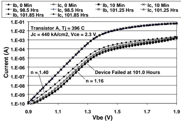
Fig. 1. Gummel plots of Transistor A measured at different stages of WLR stress. The stress current density was 440 kA/cm<sup>2</sup>.
