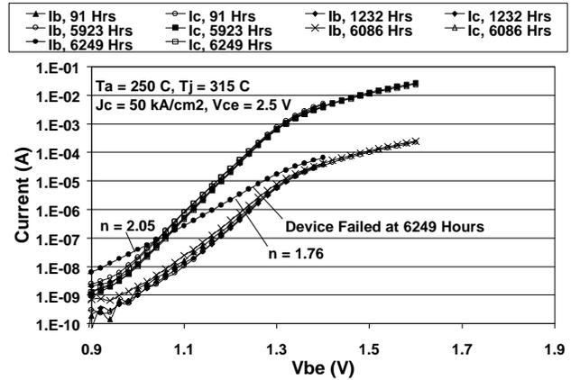
Fig. 5. Gummel plots of a  $2 \times 12 \mu\text{m}^2$  InGaP HBT measured at different stages of traditional low current stress test in oven. The stress current density was  $50 \text{ kA/cm}^2$ .
