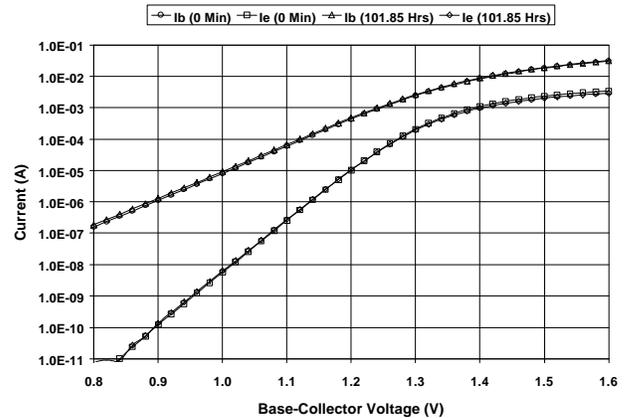
Fig. 3. Reverse Gummel plots of Transistor A before and after WLR stress. The stress current density was 440 kA/cm<sup>2</sup>.
