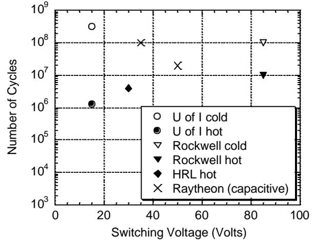
Fig. 6. Switch lifetime vs. actuation voltage for published reports
