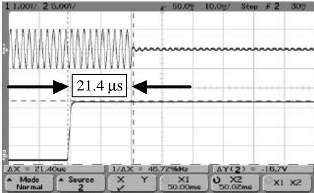
Fig. 5. Switching time data showing a delay of 21.4  $\mu\text{s}$
