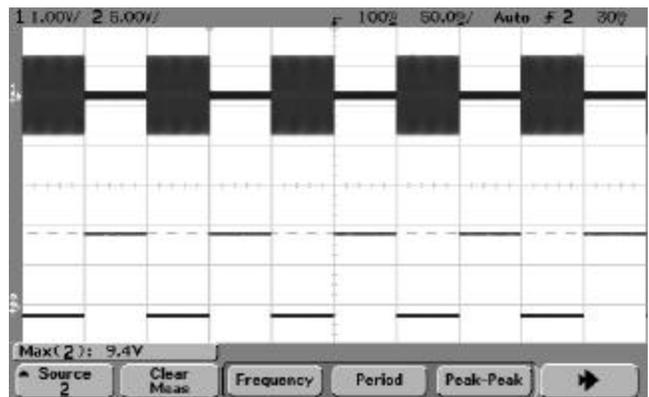
Fig. 4. Oscilloscope data for a switch operating at 9.4 Volts
