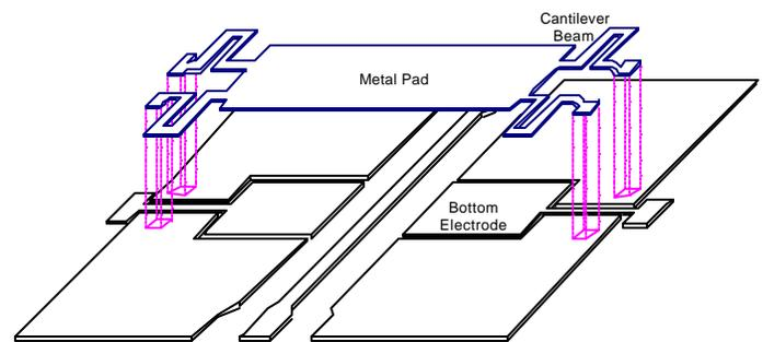
Fig. 1. Schematic diagram of an RF MEMS switch
