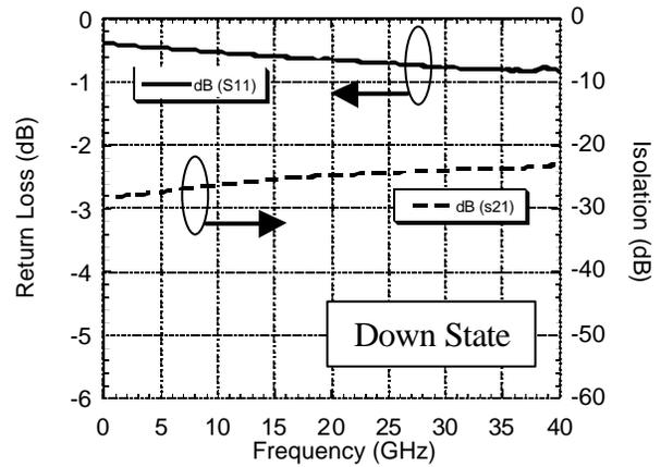
Fig. 3 (b). Measured rf performance for the down state
