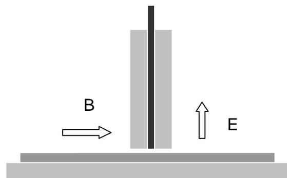
Fig 1. Schematic representation of the capacitive probe
