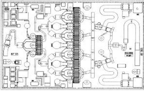
Figure 6. Layout of 11mm MMIC (TGA 9083). Die size is 4.5x3x0.1mm. Pulsed power test gave over 13 W at X-band with the new process.
