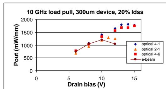
Figure 3. Load pull measurements at 10 GHz showing Pout at max PAE vs. Vd. At higher drain bias the new optical process has higher Pout than the standard process.
