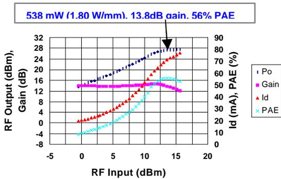
Figure 4. Load pull measurement at 10GHz of 300µm device. Tuned for power.
