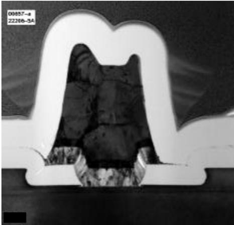
Figure 2. TEM showing finished optical T-gate defined in a layer of dielectric
