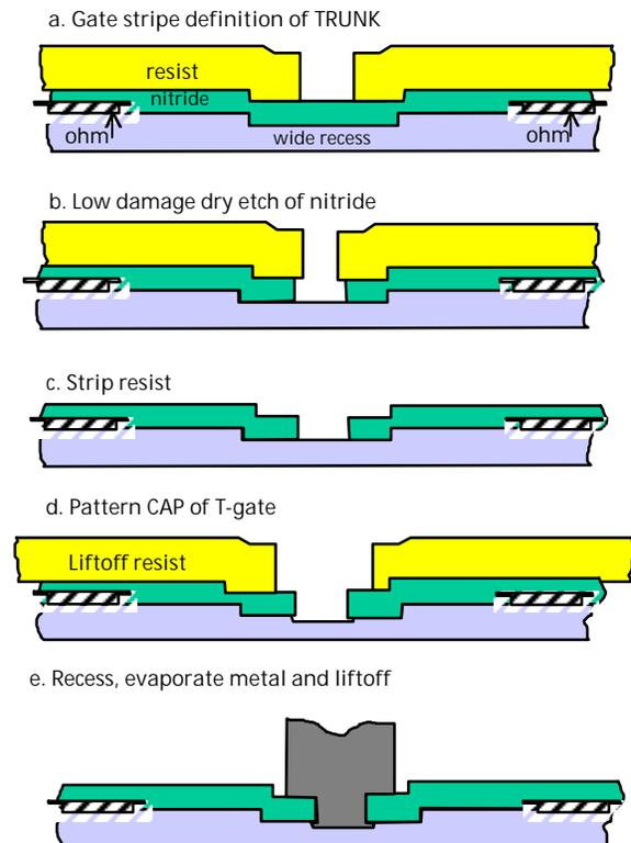
Figure 1. Diagram of process flow
