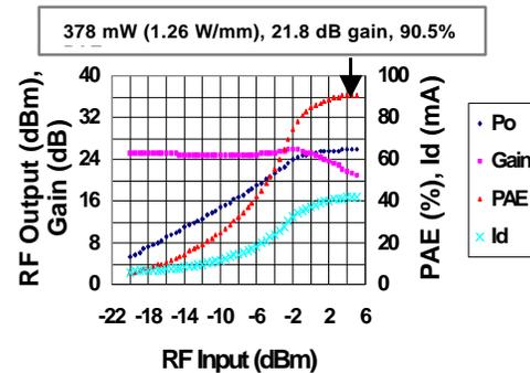
Figure 5. Load pull at 1.9 GHz of a 300µm device. Tuned for efficiency. Power tune gave over 2.0 W/mm.
