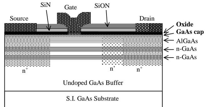
Figure 1 Cross sectional view of planer type AlGaAs/GaAs MESFET
