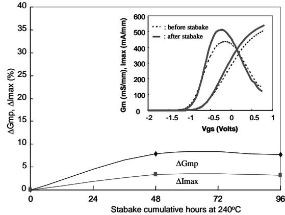
Figure 4. Thermal stability examination of HD-ICP-CVD passivated GaAs PHEMTs (Insert: recovery of characteristics of  $G_m$  and  $I_{ds}$  versus  $V_{gs}$  after stabake at  $240^\circ\text{C}$  for 48 hours).
