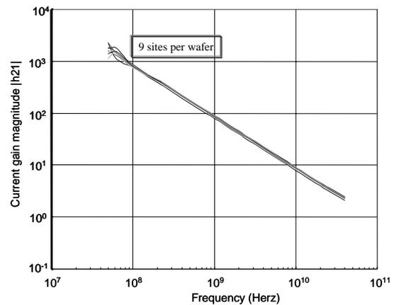
Figure 5. RF characteristics of 0.15  $\mu\text{m}$  GaAs PHEMTs passivated by HD-ICP-CVD nitrides, showing the uniform  $F_t$  distribution with a value of approximately 85-90 GHz at  $V_{ds}=2\text{V}$ .
