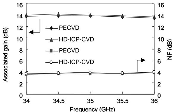
Figure 7. RF performance of a 0.15  $\mu\text{m}$  GaAs PHEMT MMIC passivated by HD-ICP-CVD nitrides, showing the comparable results to MMICs passivated by PECVD.
