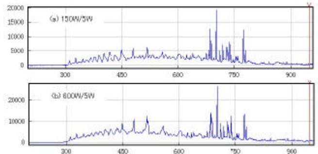
Fig.8 Plasma emitting spectra after etching of SiNx film. (a) the antenna power is 150W and the bias power is 5W. (b) the antenna power is 600W and the bias power is 5W.
