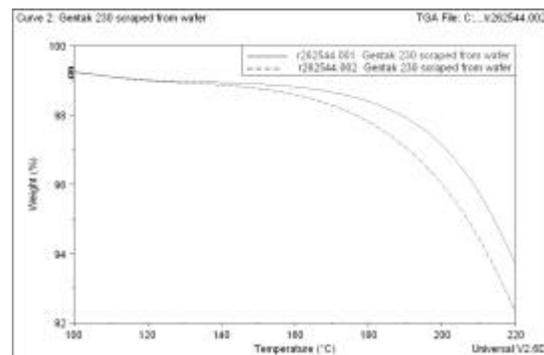
Figure 6. TGA scan of GenTak™ Indicating <0.5% at Temperatures Exceeding 130C, the Softening Range.
