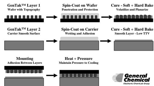
Fig. 1. Coating, Curing, and Mounting of GaAs Wafers to Non-Perforated Carriers with GenTak™ Adhesive.
