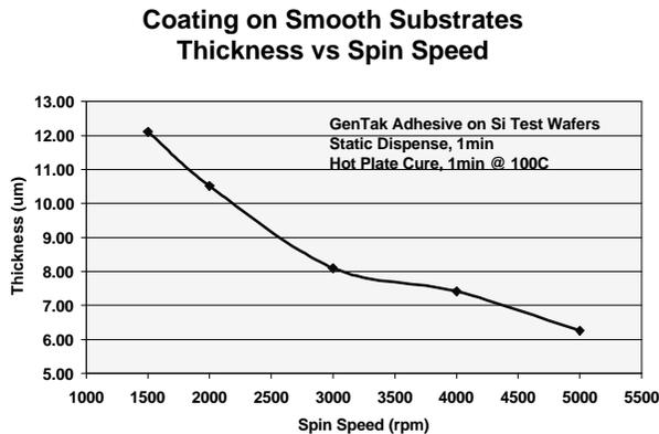
Fig. 2. Coating Thickness on Test Wafers with GenTak™ Adhesive.
