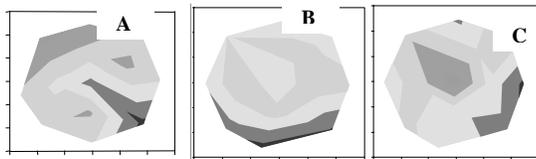
Figure 5. Contour Plots Showing Surface Uniformity of Wafer Grinding with GenTak™ Adhesive. Plots are Described: A) Bare Wafer, B) Mounted – Prior to Grinding, and C) Post Grinding. Dark Areas are Peak Thickness.
