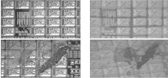
Fig. 4. Observations Through Mounted Carrier with GenTak™ Adhesive, Visible (Left Side) and the corresponding same image under UV light (Right Side). Dark Areas Suggest a Lack of Adhesive with Dye.
