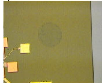
Figure 9: Frontside etch at carrier perforation
