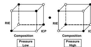
**Figure 2.** Summary of Designed Experiment. Range of factors explored and schematic of 2<sup>4-1</sup> design
