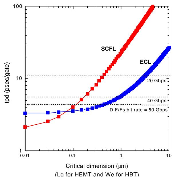
Figure 1: Propagation Delay of ECL and SCFL
