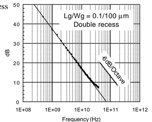
Figure 4: Cut-off frequency
