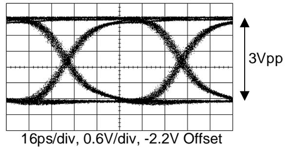
Figure 7: Output waveform of driver at  $12.5\text{Gbps}$
