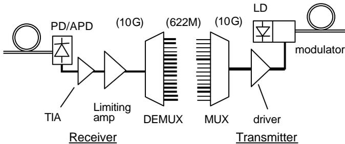
Figure 5: Block diagram of OC-192
