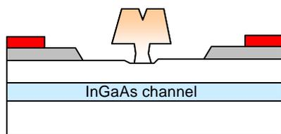
Figure 2: Recess-gate of pHEMT
