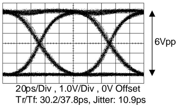
Figure 9: Output waveform of MZ driver at 10Gbps
