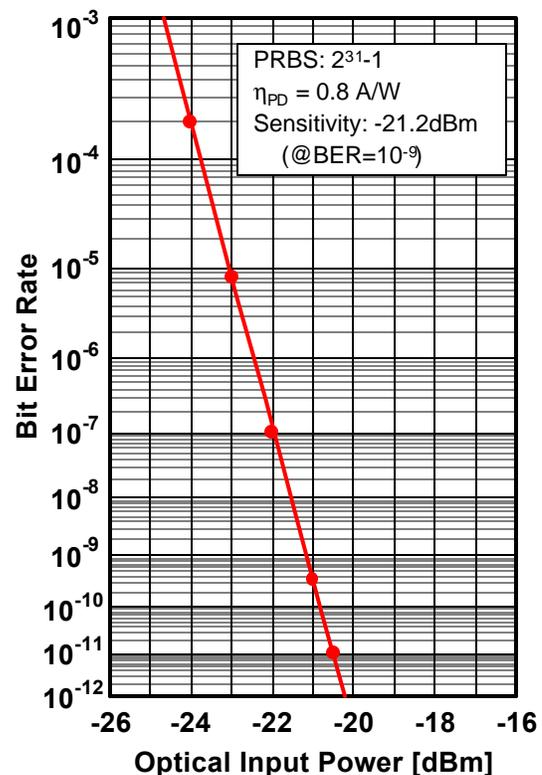
Figure 8: Bit Error Rate of TIA at  $10\text{Gbps}$
