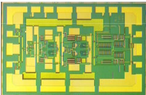
Figure 6: Photograph of driver IC
