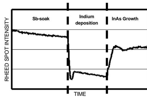
Figure 2. Reflection high-energy electron diffraction (RHEED) signal during InAs/AlSb interface formation.
