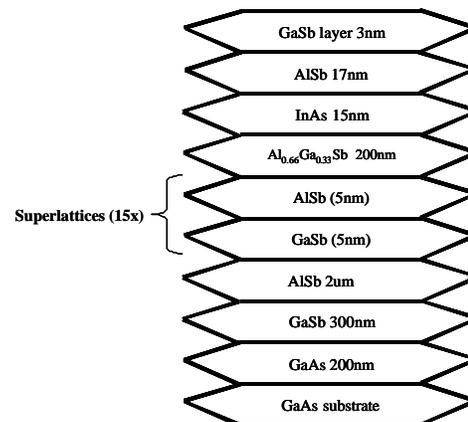
Figure 1. InAs-AlGaSb based HEMT test Structure
