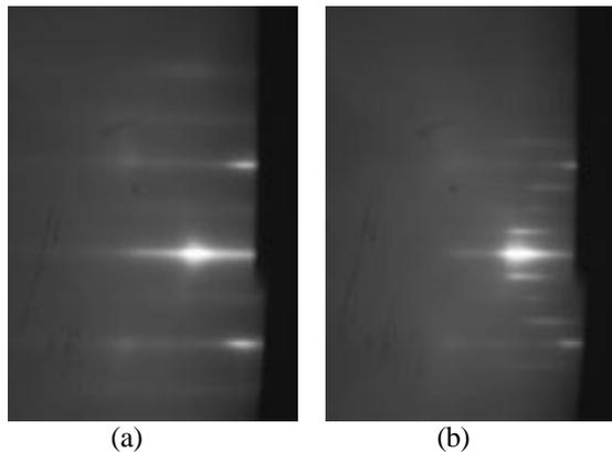
Figure 4. RHEED pattern for (a) InAs growth - “2X” and (b) Indium deposition on Sb-sublayer - “4X”
