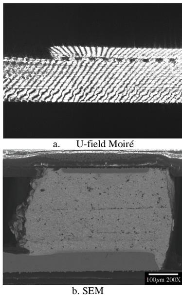
Figure 3. Solder one after 100 cycles
