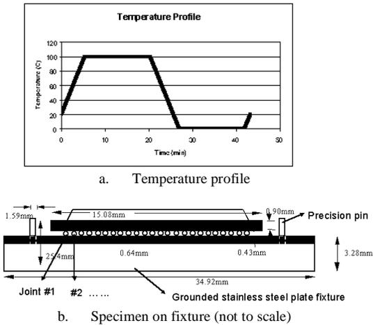
Figure 1. Temperature Profile and Specimen on Fixture
