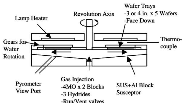
Figure 1. Schematic diagram of planetary MOVPE reactor
