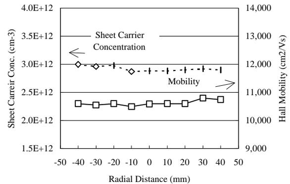
Figure 6. In-wafer uniformity of 2DEG sheet carrier concentration and Hall mobility
