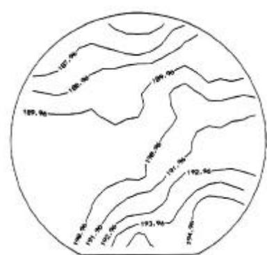
Figure 7. Sheet resistance mapping data of sheet resistance of HEMT structure without contact layer
