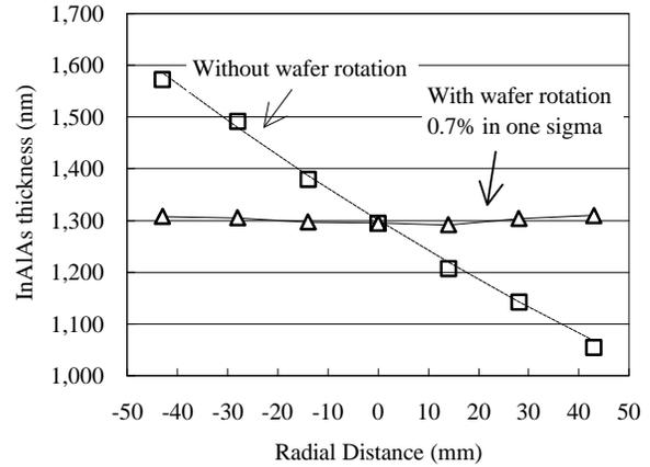
Figure 2. InAlAs thickness distribution in radial direction with and without wafer rotation. Dotted line shows fitting curve of  $\exp(-x)$  function.
