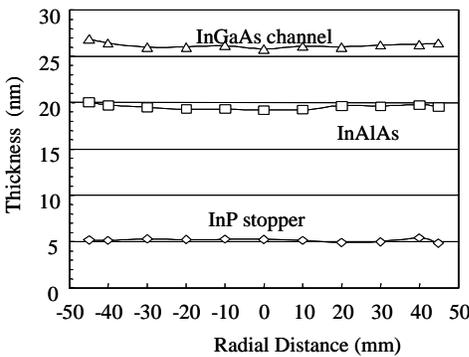
Figure 4. Thickness distribution in HEMT structure
