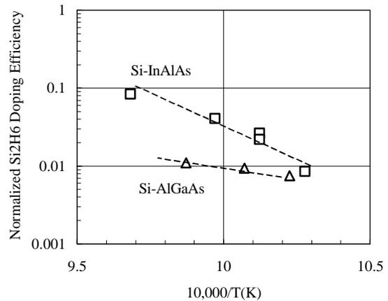
Figure 3. Arrhenius plot of normalized doping efficiency of  $\text{Si}_2\text{H}_6$  to  $\text{In}_{0.52}\text{Al}_{0.48}\text{As}$  and  $\text{Al}_{0.25}\text{Ga}_{0.75}\text{As}$ .
