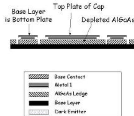
Figure 4. Schematic of Ledge CV structure
