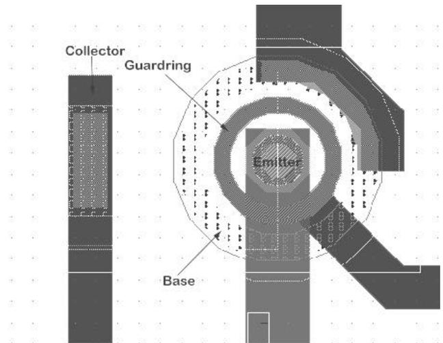
Figure 7 – Top View of Guard-ring Device
