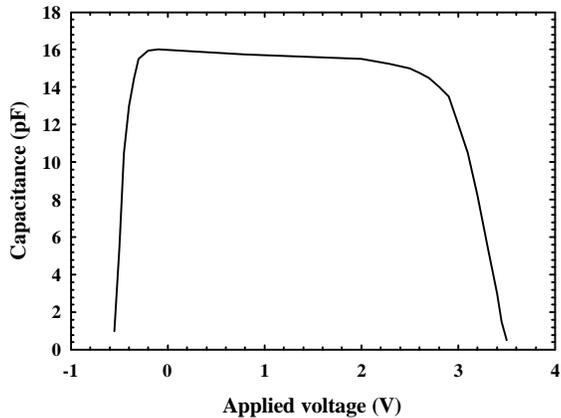
Figure 5. Data from Ledge CV measurement for 200/600 Structure
