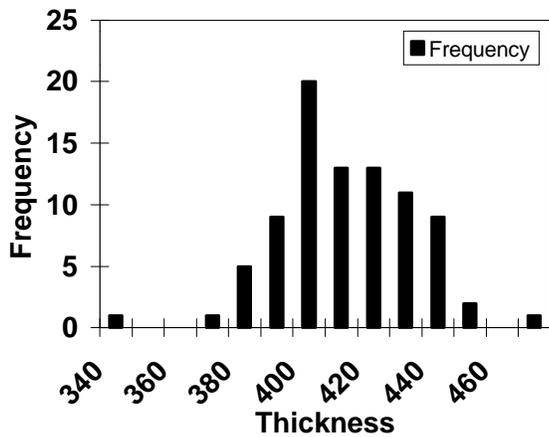
Figure 6. Ledge CV results from a single wafer lot, multiple sites per wafer. Thickness is in Angstroms
