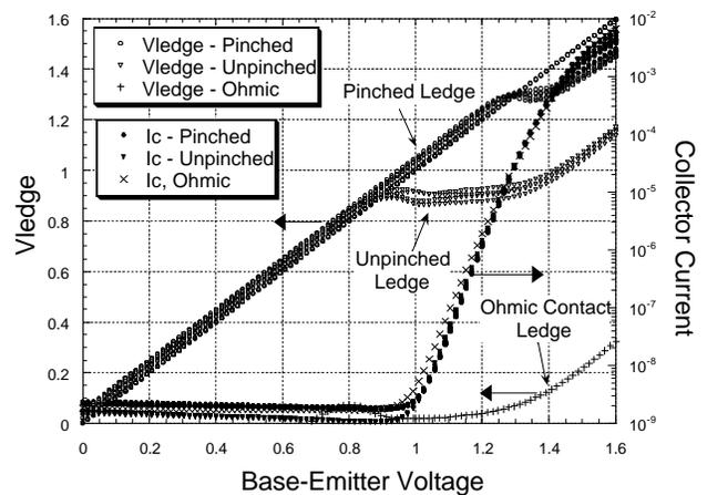
Figure 8 – Results of On-ledge potentiometer measurements.
