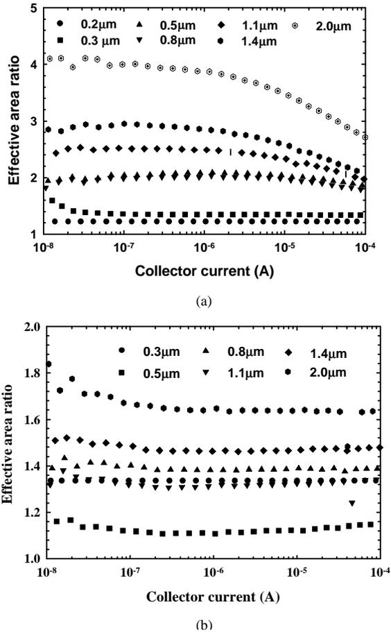
Figure 2. Examples of Effective Area Ratio Measurements for 4  $\mu\text{m}^2$  devices
