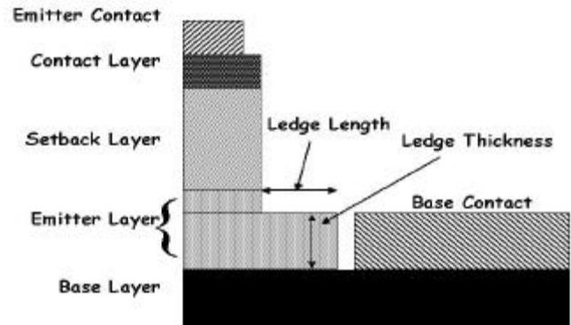
Figure 1. Schematic Of Ledge Region of an HBT
