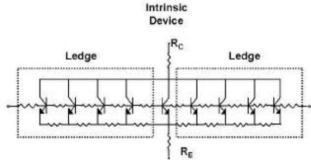
Figure 3. Equivalent circuit representation of HBT with ledge
