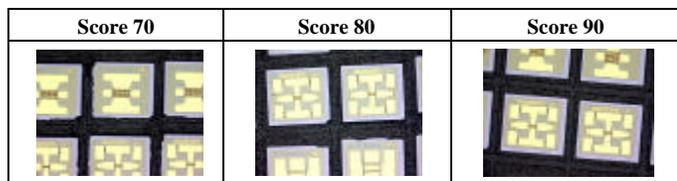
Figure 6 Visual inspection with a score system for scribe & break
