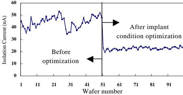
Figure 3 Great improvement in leakage and uniformity after DOE
