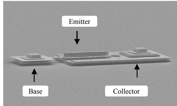
Fig. 2. A fabricated InP/InGaAs HBT before planarization
