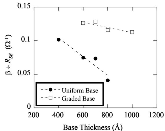
Fig 1.  $\beta \div R_{SB}$  as a function of base width for uniform and graded bases.
