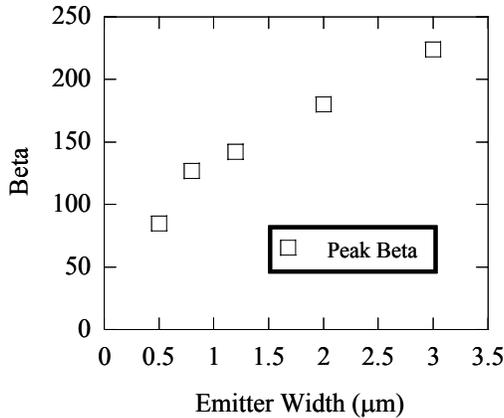
Fig 4. The decrease in  $\beta$  with emitter width. The emitter length of all devices was 12  $\mu\text{m}$
