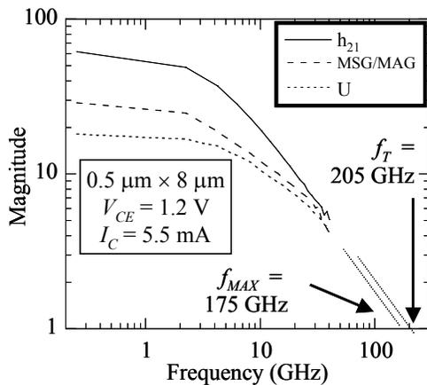
Fig 5. Example extrapolation of  $f_T$  and  $f_{MAX}$
