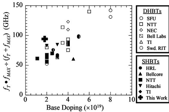
Fig 9. InP HBT RF performance measured with a single parameter derived from  $f_T$  and  $f_{MAX}$  vs. base doping in technical literature.
