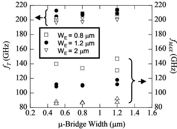
Fig 8. RF performance vs.  $\mu$ -bridge width. The emitter length of all devices was 12  $\mu\text{m}$ .
