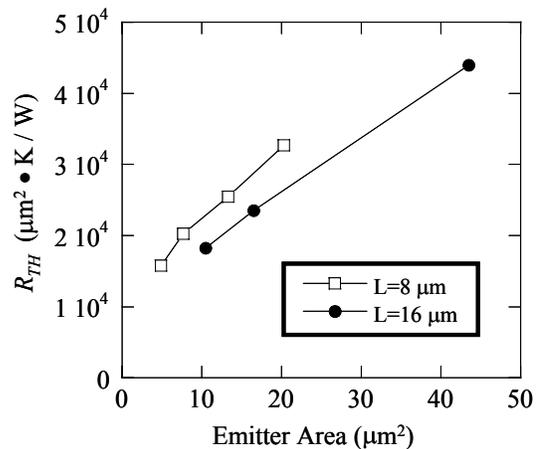
Fig 7. Area-normalized thermal resistance for different sized devices.
