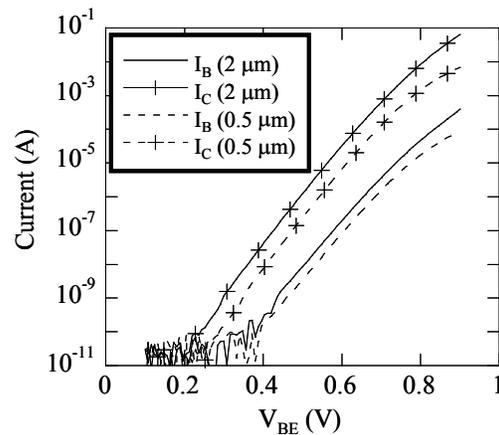
Fig. 3. Gummel plots for two fabricated devices. The emitter length of both devices was 12 μm
